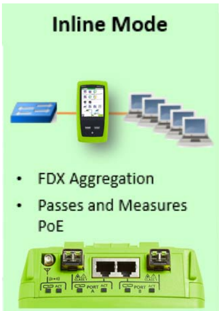
Figure 19. Inline packet capture simplifies documentation of client application problems without TAPs or SPAN ports
