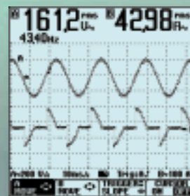
Dual-input measurement shows both meter reading and waveform at the same time.
