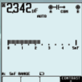
Check the starting capacitor of a motor with the ScopeMeter 120 Series.
