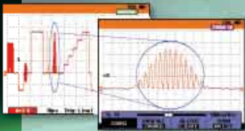
Thanks to the deeper memory, very small parts of the waveform can be studied in full detail using 'zoom'.
